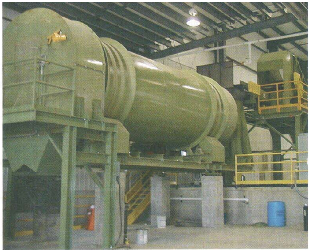
After passing through a picking line to remove contaminants, materials are conveyed into a large mixer, along with water, wood chips, soiled paper, pasteboard and cardboard.
