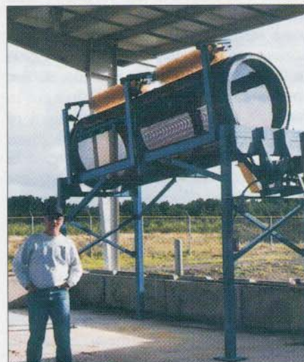
Mixing augers shred and blend the mix of compostable material and bulking agent.
