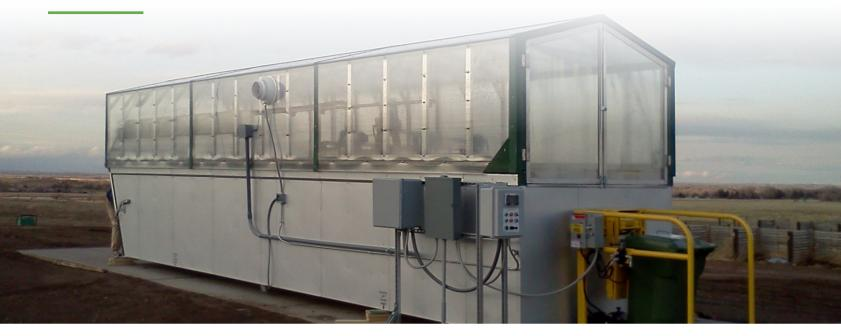
The Earth Flow Custom Vessel system is built within a stainless steel, greenhouse roof enclosure for heat gain and odor control. The award-winning Earth Flow automated auger mixing system both shreds and aerates the compost while moving the material toward the discharge end of the vessel and requires little labor beyond loading and unloading. The Earth Flow provides control of odors while making gorgeous compost.
