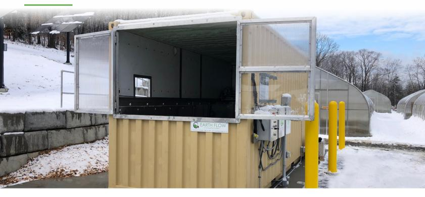
The Intermodal is a re-purposed shipping container that lowers the cost of the in-vessel Earth Flow system by up to 40%. The Earth Flow  $^{\text{m}}$  is equipped with a fully automated mixing, aeration and moisture addition system for optimal compost process management and odor control. The shipping container is lined with insulation and stainless steel for a long service life.
