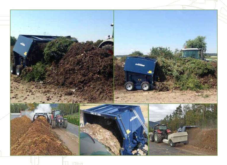
With a rotor length of 3.5 m and a heap cross-section of about 4 m², Compost Systems expands its Agroline with the CMC ST 350 for tractors above 100 hp. With or without a super creeper gear, the CMC ST 350 works well with a push axle (option) even without creeper speed. The turner has a transport height of more than 4.6 m, which is not suitable
