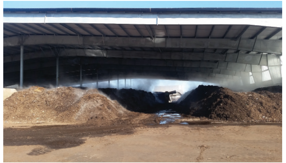
The Enviro-Smart composting facility in Delta, B.C. uses a fully automated high-pressure negative aeration sparger floor to aerate curing compost.
